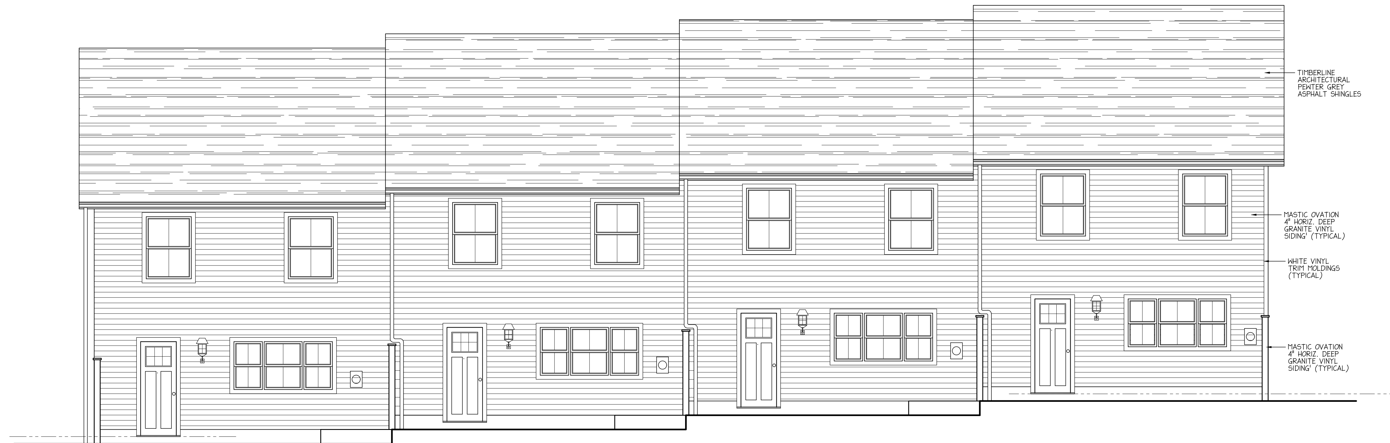
1 PROPOSED REAR ELEVATION 1/4" = 1'-0"
