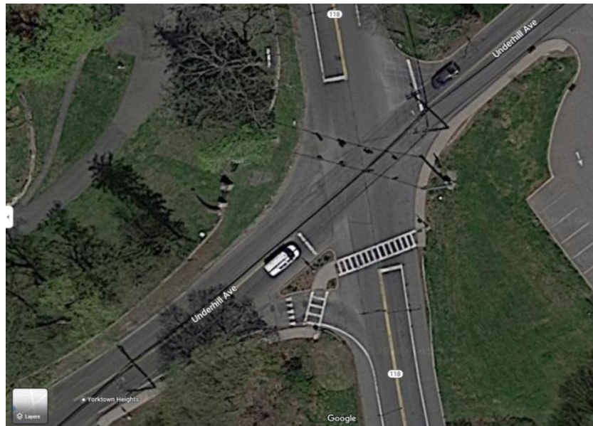
Figure 1: Aerial photography showing channelized right-turn of eastbound Underhill Avenue approach to NY 118 (source: Google Maps)
