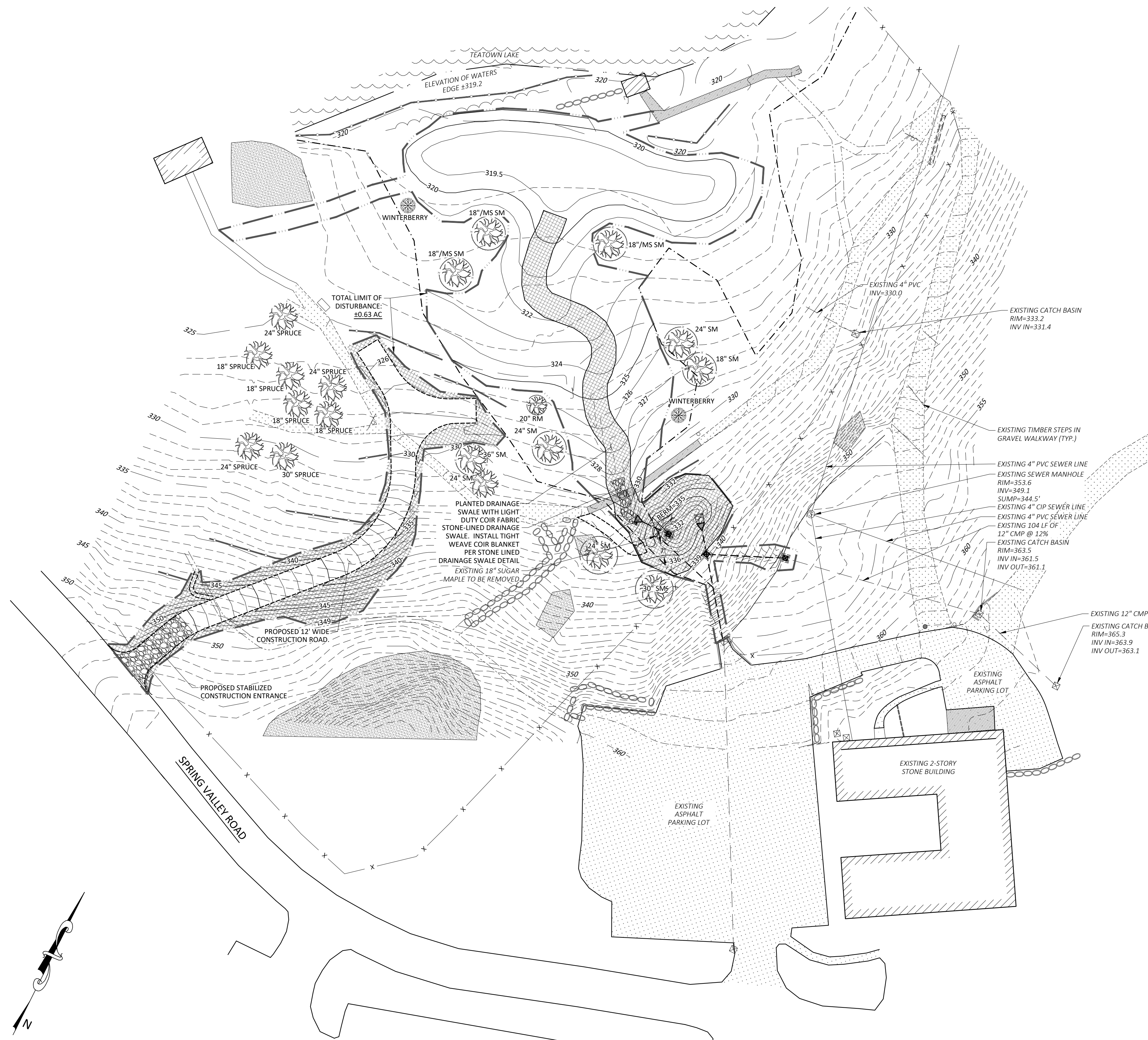
1 PROPOSED EROSION AND SEDIMENT CONTROL PLAN C-2 SCALE: 1"=30'
